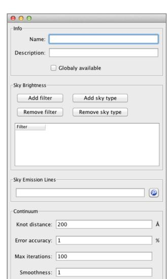
A new plugin to build a sky brightness depending on the phase of the moon has been integrated. It uses brightness tables to create the overall brightness of the sky. It includes the possibility to add filter measurements with errors and define several types of the sky (bright, grey, dark or any other label you might want to put).
