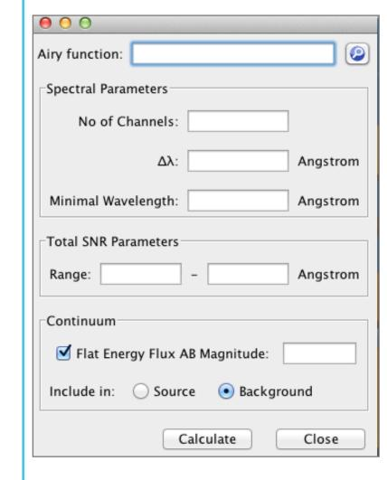
A new plugin has been developed to deal with Fabry Perot observations. This plugin allows to compute the signal to noise ratio of an observation on a tuneable wavelength interval. The plugin has specific inputs like the finesse, the wavelength range (or the number of channels combined with the wavelength bin in Å).
