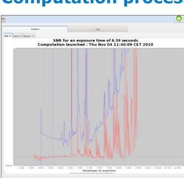
Results are displayed in the interactive plot window with respectively the signal to noise ratio distribution, the output signal and the noise contributions.
